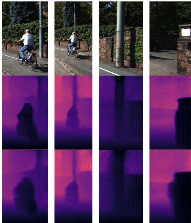
Fig. 1. Comparison of depth prediction results with (second row) and without (third row) a z-buffer in the self-supervised training pipeline. Differences are most pronounced at large depth boundaries where occlusions are most prominent. (Images from the KITTI [1] Eigen test split.)
